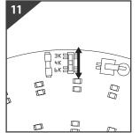
Use the CCT selection switch on the gear tray to select the desired colour temperature
