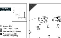
Connect battery pack cable to lamp panel
