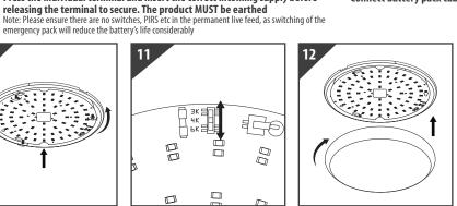
Push and twist the diffuser back into place
