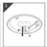
Pull power supply through hole in the base plate
